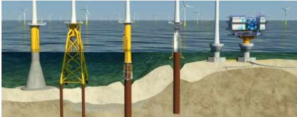
Figure 2 Illustration of offshore wind farm foundations designed by COWI. From left: Thornton Bank Concrete, Wikinger Jacket, 2* London Array Monopiles, Nysted Concrete, Rødsand 2 Offshore Substation
