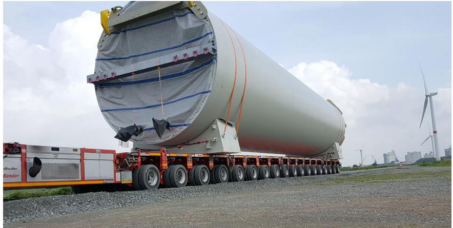
Figure 6-5: SPMT for transportation of large heavy components
